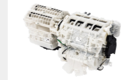
Smaller and lighter air-conditioning units that can be installed across manufacturers, car models, and powertrains
