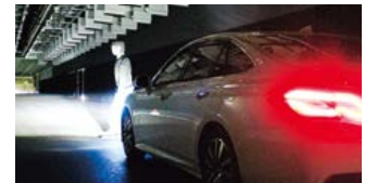
A nighttime pedestrian model used in our assessment of collision avoidance braking systems
