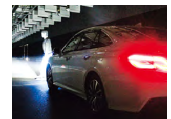
A nighttime pedestrian model used in our assessment of collision avoidance braking systems
