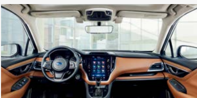
Integrated cockpit system (center display, combination meter, HMI control unit) Instrument panel inside a Subaru Legacy
