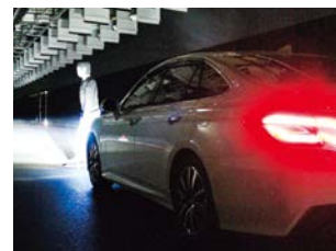
A nighttime pedestrian model used in our assessment of collision avoidance braking systems
