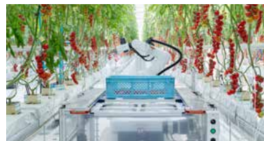
Cherry tomatoes harvested by an automated harvesting robot
