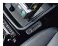
Separate switch for the air purifier
