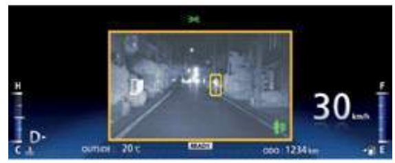
Night View System with Pedestrian Detection Function
