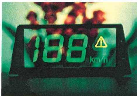
Fig.9 An example of the green-amber multicolor transparent EL display applied to a head up display.
