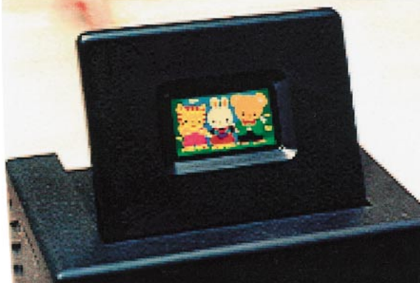
Fig.12 An example of the 1.8-inch-diagonal RGB 18-color EL display with the dual panel configuration.
