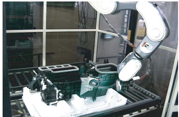
Fig. 19 Appearance of inspection system for automobile air conditioner
