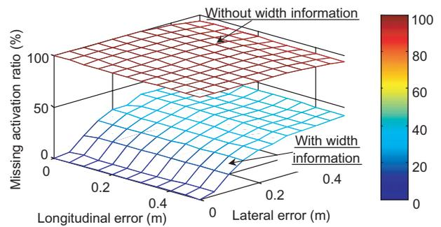
Fig. 11 Missing activation ratio on 0.1m lap collision
