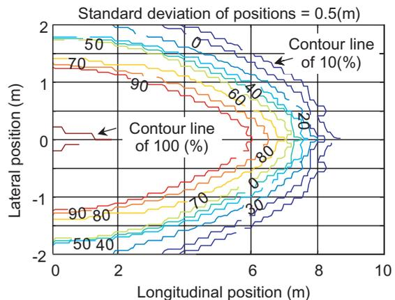
Fig. 10 Examples of collision probability map
