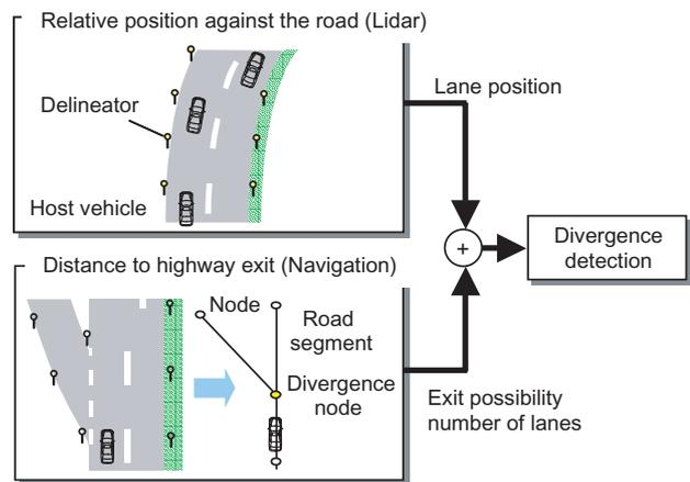
Fig. 6 Outline of divergence detection algorithm
