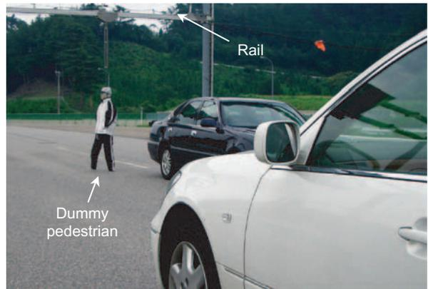
Fig. 4 An example of test scenario and facility for pedestrian sensing test
