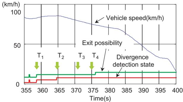
Fig. 7 An example of divergence detection result
