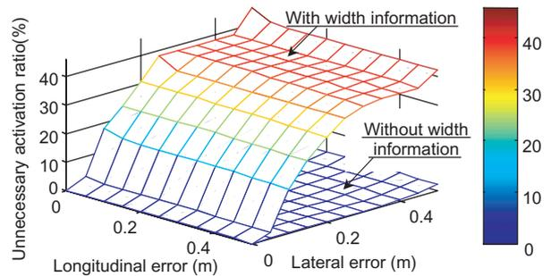
Fig. 12 Unnecessary activation ratio on 0.1m gap passing
