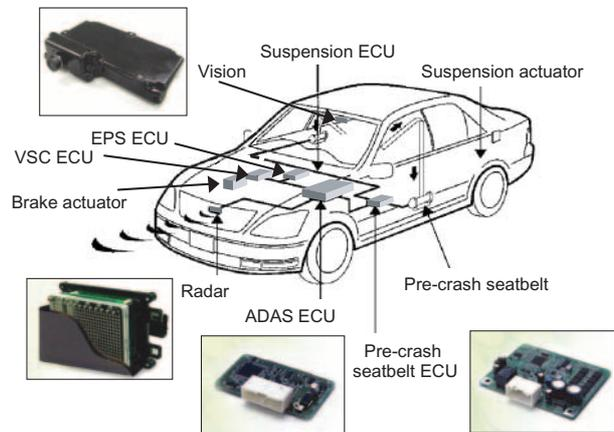
Fig. 2 An example of ADAS configuration
