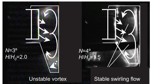
Fig. 10 Visualized flow in the various type of expanding scroll casing ( l/D=0.16 )
