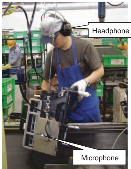
Fig. 1 Inspection by person
