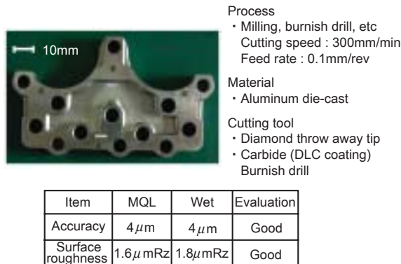
Fig. 12 Real application example of aluminum use cutting fluid (Sensor board plate)
