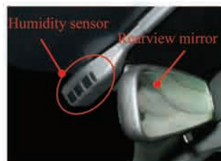
Fig. 5 Appearance of Sensor Installed on the Front Windshield
