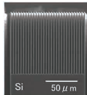
Fig. 2 Sectional SEM Photograph of the Silicon Substrate after Etching
