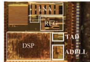
Fig. 8 Photo of 0.18 μm RCC Receiver IC (active area: 1.8 mm 2 )
