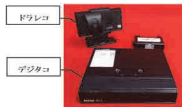
Fig. 15 Digital tachograph and drive recorder that has been commercialized
