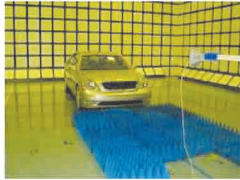
Fig. 17 Vehicle Antenna Measurement in Radio Anechoic Chamber
