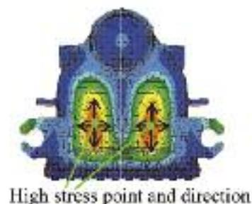
Fig. 5 Stress distribution of intercooler tank
