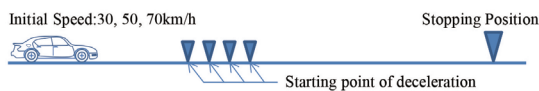
Fig. 1 The relationship of the initial speed, starting point of deceleration, and stopping position
