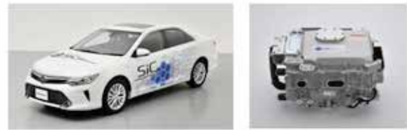
Fig. 3-7 View of the test car and PCU installed SiC MOSFET 17)
