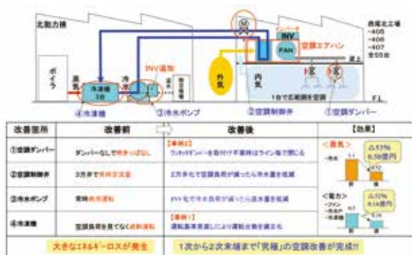
Fig. 8 AC Air-Handling Unit Energy Use Improvement
