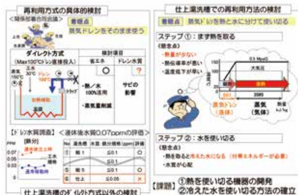
Fig. 3 Steam Drain Obstacles to More Efficiently Using Heat and Water
