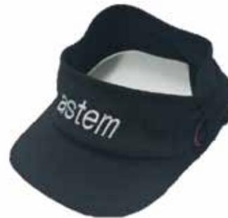
Fig. 3 Wearable NIRS system (Sun visor-type)
