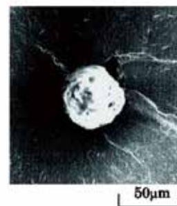
Fig. 4 Inclusion observed at fracture origin (Murakami et al., 2000a)
