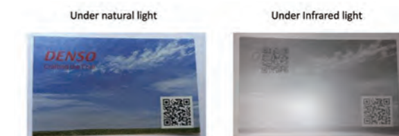
Fig. 8 Transparent QR code. The public QR can be seen at the bottom-right corner. The private QR was hidden under DENSO logo
