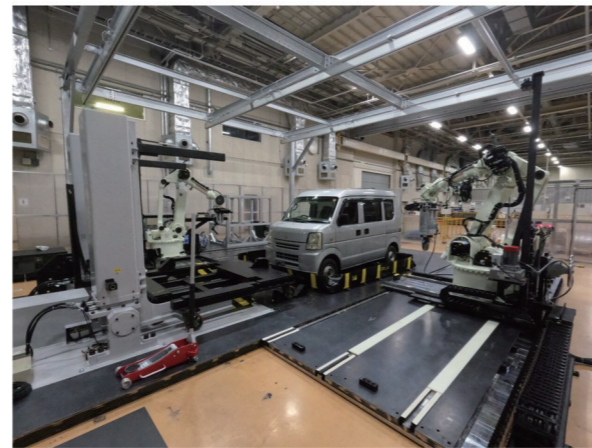
Fig. 4 ELV Disassembling laboratory
